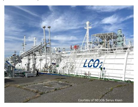
JCCS started a demonstration test using the TBG loading arm in Tomakomai on October 7-9. This demonstration test was conducted under lower temperature and pressure conditions than typical liquefied CO2 transport conditions (-20°C or lower, 2.0 MPa or lower).
