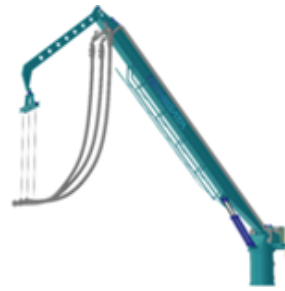
Ammonia bunkering boom (3D model)
