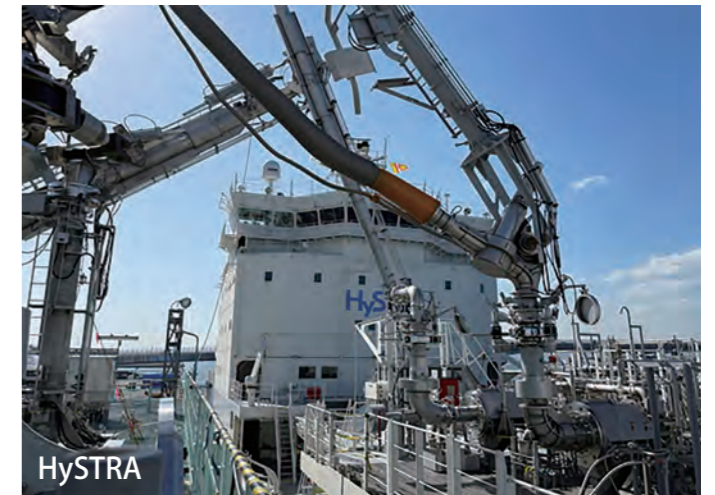
Loading/Unloading operation of 6" LH2 Marine Loading Arm
